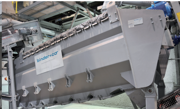
Binder+Co de-labelling machine
