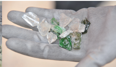
Glass after optical sorting
